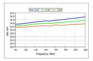
Figure 8. Idd vs Frequency
