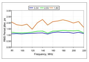
Figure 9. RMS Period Jitter vs Frequency
