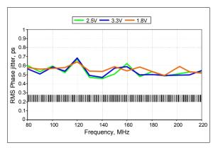
Figure 11. RMS Phase Jitter vs Frequency
