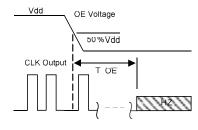
T\_ $\overline{OE}$ . Time to put the output drive in High  $\angle$  mode
